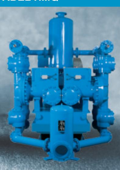
ABEL hydraulic membrane pumps take full advantage of modern membrane technology. They are equipped with pre-formed membranes and pressure-balanced membrane positioning that stabilises pressure and flow for the membrane movement between the front and rear limit of stroke. Unlike most other membrane pumps, ABEL Series HM membranes are not stretched during the stroke. This ensures longer membrane service life and more dependable operation.
