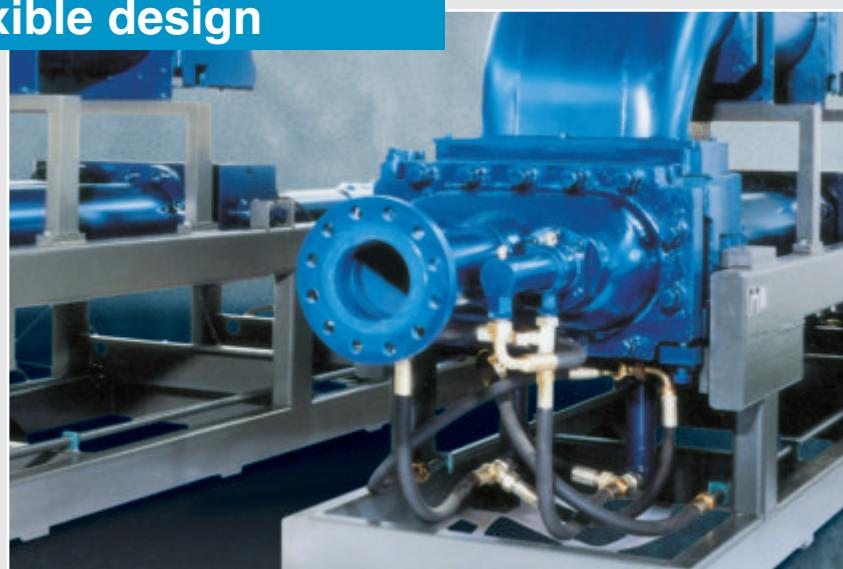
Even non-newtonian media are included in the wide spectrum of materials transferred by Positive Displacement Pumps.
